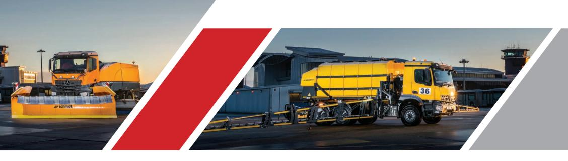
Designed specifically for keeping runways clear and ice-free, the ASP is available as both a fix-mounted or demountable variant for trucks, operating at speeds of up to 30mph and with spraying widths ranging from 3-30m.
